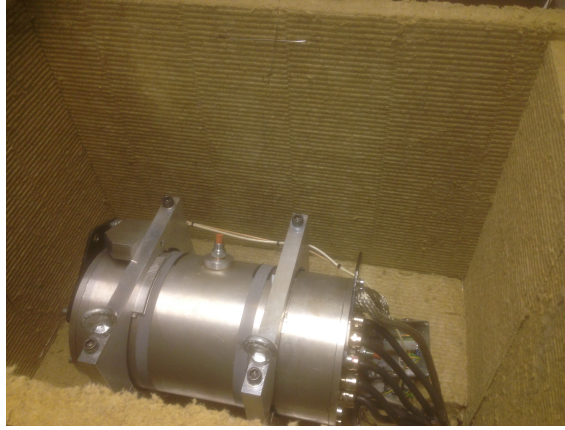
Figure 5.15: The PMSM placed inside an isolated cage for the purpose of investigating thermal dependency.
