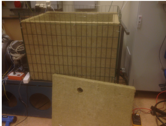
Figure 5.16: The isolated cage containing the PMSM.
